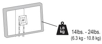
Total weight of monitor when mounted needs to be 14 lbs - 24 lbs (6.3 kg - 10.8 kg)
