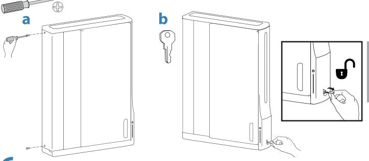
a. Open door and remove these 3 screws. Save screws for reattaching cover.  $\overline{}$ b. Remove left cover
