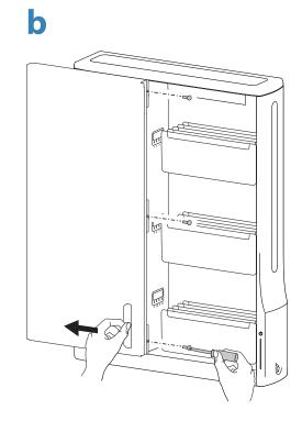
a. Close door and turn lock knob 180° counter clockwise.b. Lock door by turning key 180° counterclockwise.
