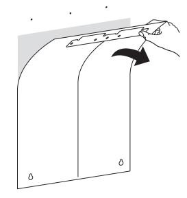
Insert anchors into holes, then attach mounting bracket. Verify wall bracket is level before tightening screws.
