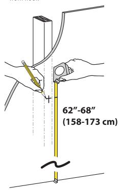
Place template on wall lining up the chosen hole with the stud and the mark 62"-68" (158-173 cm) from floor.
