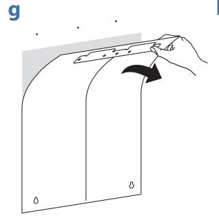
Insert anchors then attach bracket to wall according to the hole option determined on previous page. Verify wall bracket is level before tightening screws.
