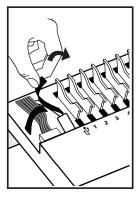
Unplug the USB and DC power cables (push up on the lever under the DC connector to release). The drawer can now be removed.
