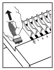
Unwind and remove any USB cables that need to be replaced.
