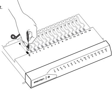
Place the drawer upside down and route the USB cable through the slot on the back of the drawer and under the hooks toward the front. Make sure there is no slack in the cable. All excess cable should hang from the hooks.
