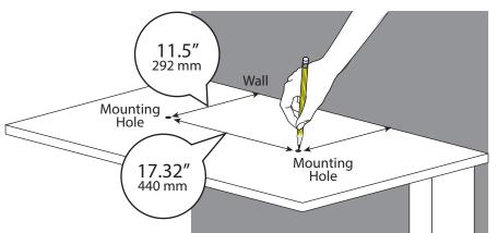
3 Drill two mounting holes using a 0.266 OD drill bit.
