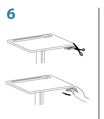
Lift brake release lever to raise and lower riser.
