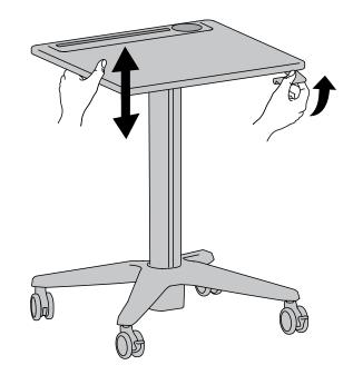
8 Loosen, but do not remove 2 screws to lift and lower hook to desired height.
