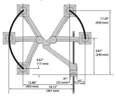
Top view showing range of motion when pulled out from the wall.
