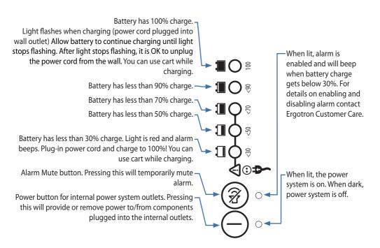
NOTE: Frequent operation of the cart while battery charge levels are below 30% will significantly reduce the life of your battery.
