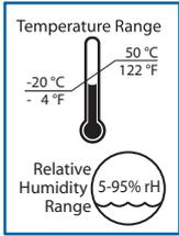
• The recommended cart storage temperature is 25°C (77°F). At this temperature, the battery's age-related capacity loss is minimized. The minimum storage temperature is -20°C (-4°F) and the maximum storage temperature is 50°C (122°F). The recommended humidity range for storage is 5-95% rH.
