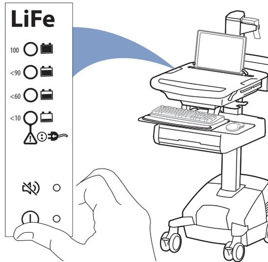
**c** With cart's power cord plugged into the wall outlet, wait until cart is at 100% charge. (takes approximately up to 2.5 hours to charge)
