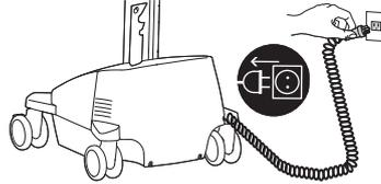
**c** Turn power system off by holding down the AC Outlet Power button for 1 - 3 seconds. Power light will shut off.
