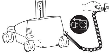
**3** Turn power system off by holding down the AC Outlet Power button for 1 - 3 seconds. Power light will shut off.
