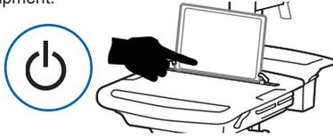
**2** Plug power cord into appropriate wall outlet to fully charge battery to 100% (all indicator lights will be illuminated). Power system must be fully charged before storing!
