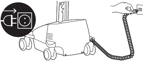
Do Not stretch coiled cord further than 8 feet (2.5 meters), damage to the cord may occur.
