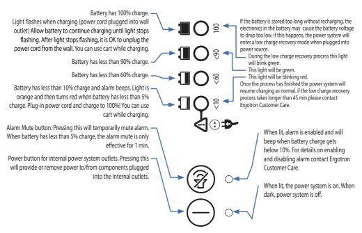
If other lights are flashing red/green it could indicate a power system fault. If this occurs contact Ergotron Customer Care.
