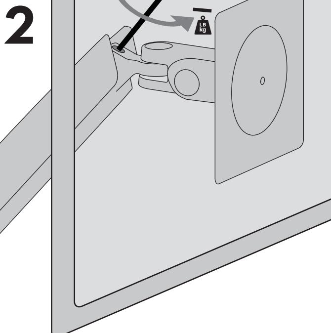
**CAUTION: DO NOT overtighten fasteners. Overtightening may cause damage to your equipment.**
