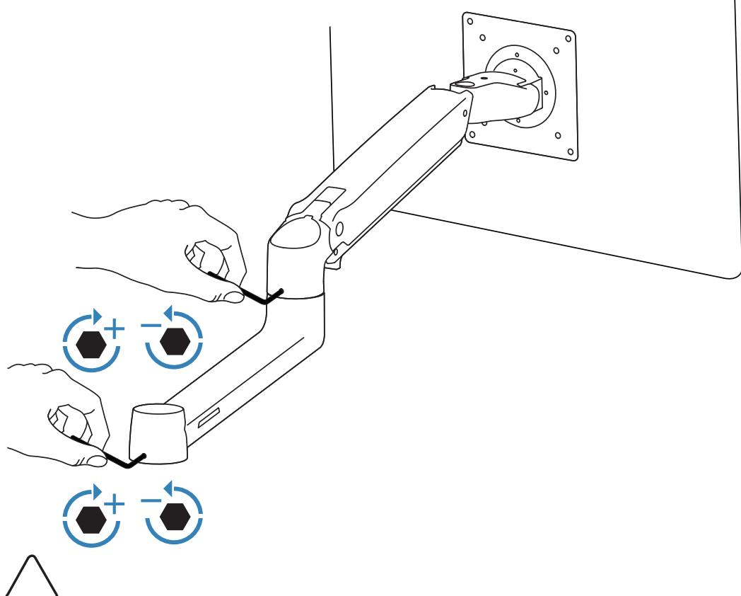
**CAUTION: DO NOT remove screw. Removing screw may cause damage to equipment.**
