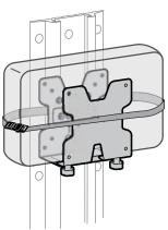
a. Attach Thin Client to brackets. Secure Thin Client.
