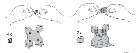
Mark mounting holes in desired location using bracket shown.
