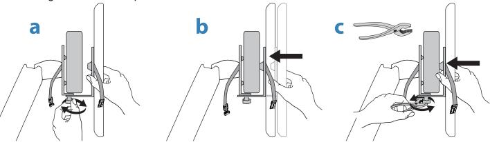
If you are using the strap and buckle, clip buckle together and tighten strap.
