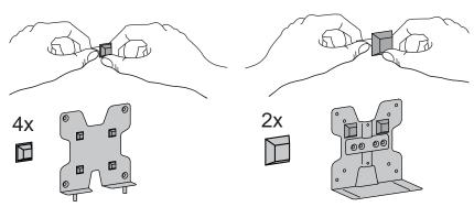
Attach bracket shown to Wall Track bracket.
