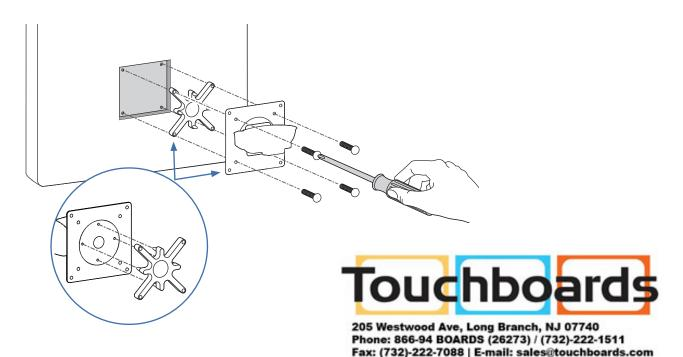
a. Remove the top, left screw and discard. (If using spacer, do not discard the screw!)
