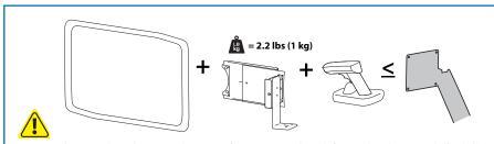
CAUITON: Make sure you know the max. weight capacity of your mounting solution before attaching the scanner shelf. Include the weight of your monitor, scanner shelf, scanner base and scanner: when figuring mounted weight on your mounting solution. Failure to follow this Caution may lead to equipment damage and/or personal injury.
