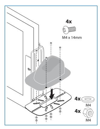
Keyhole mount: attach interface plate to L-bracket using 1 washer and 1 nut, then attach scanner base using 2 shoulder screws, 2 washers and 2 nuts.
