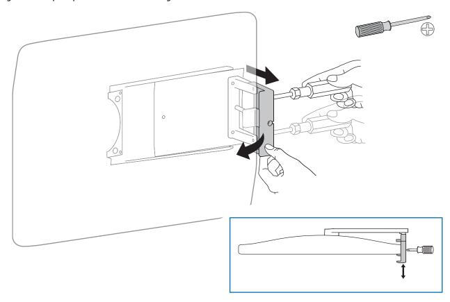
Tighten the front screw until the spacer holds the display snug.
