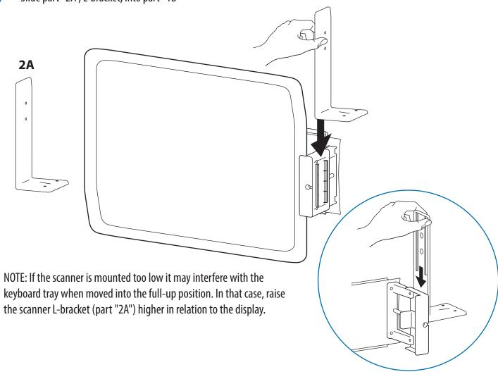
Adjust the L-bracket to desired height and tighten screws with a flat-head screwdriver.
