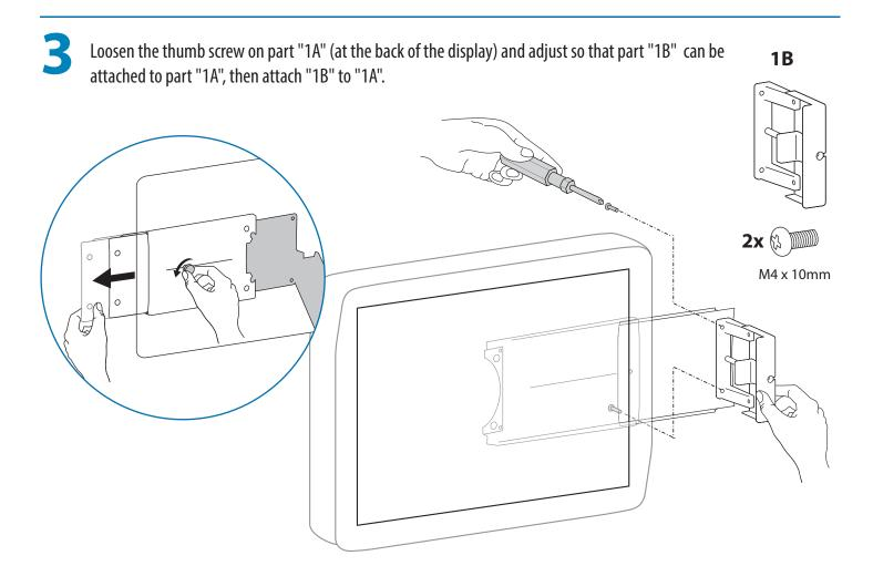
Loosen the thumb screw on part "1A" (at the back of the display) and adjust so that part "1B" comes into contact with the side of the display.
