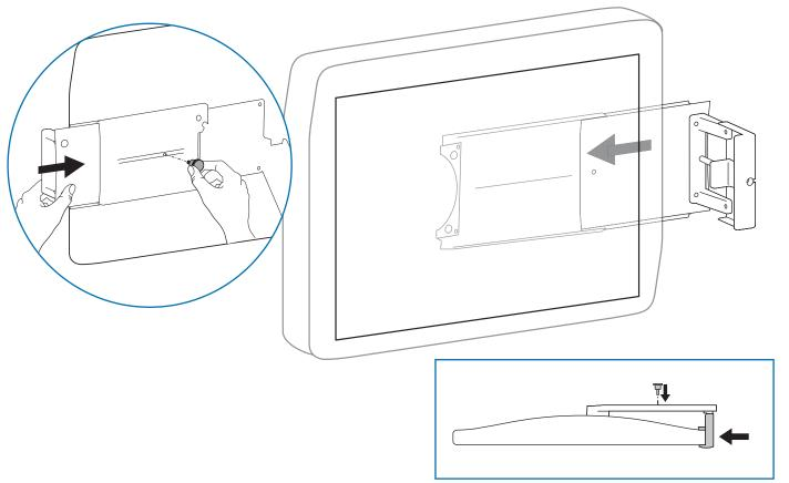
Pull the front section of part "1B" forward so that it grips the front of the display. Tighten with phillips screwdriver until snug.
