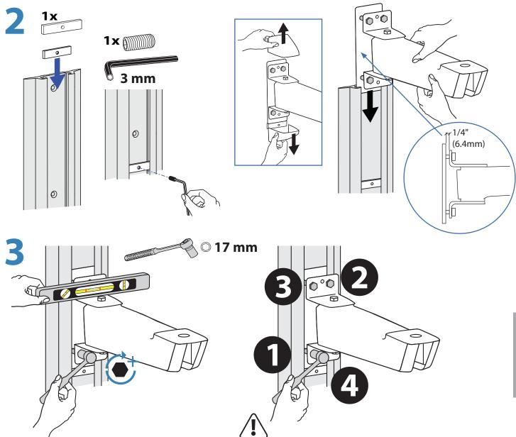
IMPORTANT! Torque bolts in the sequence shown above to a minimum of 50 lb-ft (6.91 kgf-m).
