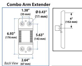
Mounting height assumes there is a 6" (152 mm) distance between the center of your monitor mounting holes and the top of the screen. If your distance is smaller, you should increase mounting height accordingly, if your distance is larger, you should decrease your mounting height accordingly.
