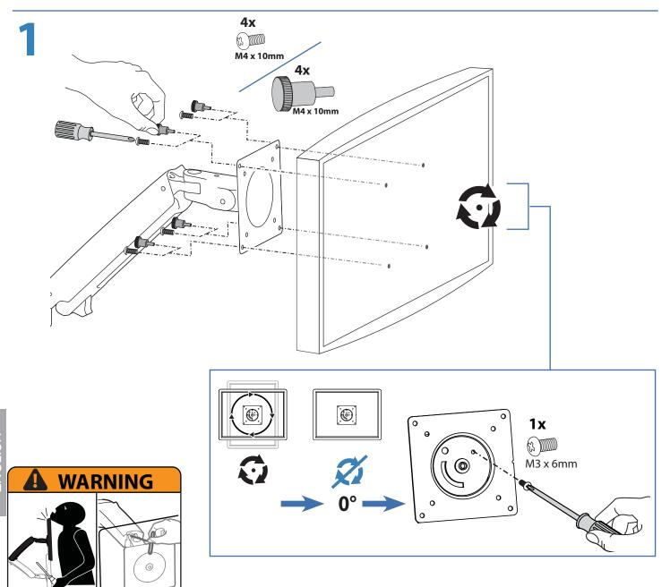
WARNING! Stored Energy Hazard: The arm mechanism is under tension and will move up rapidly, on its own, as soon as attached equipment is removed. For this reason, DO NOT remove equipment unless the arm has been moved to the highest position! Failure to follow this instruction may result in serious personal injury and/or equipment damage!
