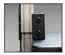
**Step 11:** Attach black end cap using the (2) 1/4-20 x 3/8 Button Head Cap Screws. Gently tighten with the 5/32 allen wrench.
