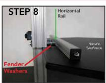
**Step 8:** Lift the Work Surface up and align the holes in the Horizontal Rail with the (2) 1/4-20 x 3.50 Hex Head Bolts{B}. Push the Work Surface onto the Hex Head Bolts until the threads of the bolts come through the Horizontal Rail.
