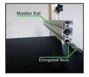
**Step 10:** Position one of the black shelves as shown. Have the elongated nuts loose and in line with the bottom channel of the monitor rail. Slide the elongated nuts into the monitor rail to you desired position and then tighten the bolts using the 7/16 wrench. Attach both shelves this way.
