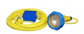
• Lightweight, Impact-Resistant Nylon Housing.• Impact-Resistant, High-Temperature Lens.• Large rubberized cushion. • Ergonomic Handle • Outdoor/Wet Location rated. • Heavy duty SOOW cord. • Designed for confined space applications. • Rugged low voltage LED Technology• 50,000 Hour Lamp Life • Cool, Glare Free Lighting• Rubberized, sealed in-line transformer assembly, converts 120V to 12VAC.
