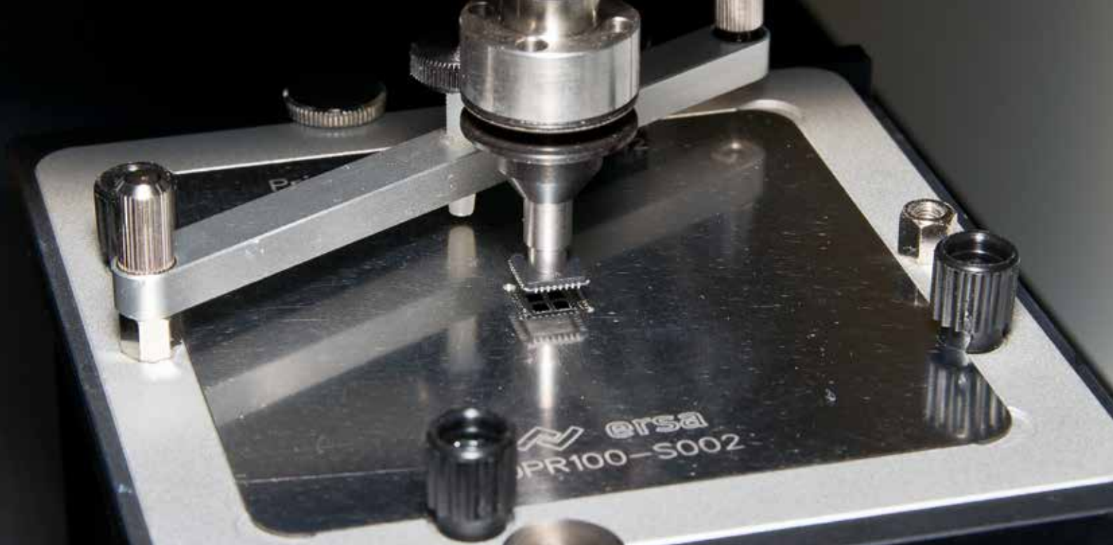
Component is lifted off the print stencil
