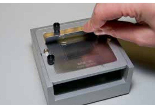
Flux application in a dip stencil
