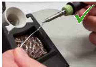
Add new solder after cleaning
