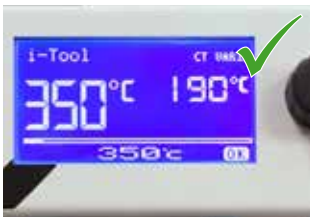
340 – 360 °C for lead-free solder
