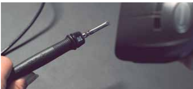
Process data documentation - the connectivity of the i-CON TRACE allows the documentation of every single soldering process: Assembly, tip used, temperature and soldering duration are recorded electronically and can be traced. Left picture: Scanning the QR code of the soldering tip with the hand-held scanner before soldering.
