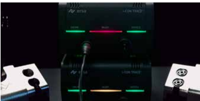
Unique operating concept: GREEN MEANS GO. Once all the requirements for the assigned soldering task have been fulfilled, the LED interface of the i-CON TRACE literally switches to green and the user can start the soldering process.
