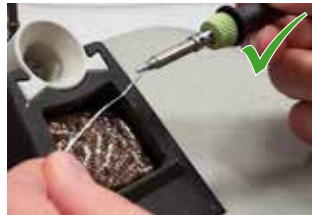
Add new solder after cleaning
