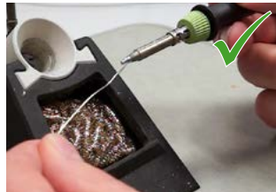
Add new solder after cleaning
