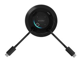
When pressing another touch button on a connected port the screen sharing will switch to the other device. The light in that section will turn blue and the light will turn off in the other sections.
