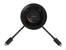
When pressing another touch button on a connected port the screen sharing and the connected equipment will switch to the other device. The light in that section will turn red and the light will turn off in the other sections.
