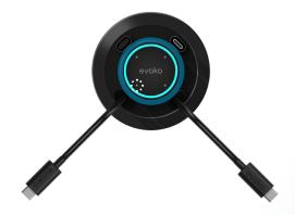
If you want to switch back to HDMI-Ingest you can long-press any button for 2 seconds. The circle will pulse blue a couple of times to indicate the mode switch and the he MTR-device will take over control of the cameras, speakers and microphones. You will still share the screen.
