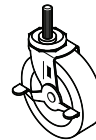
3" Locking casters (set of 4), 2 locking, 2 non-locking ( \frac{3}{16} "-18 x \frac{3}{4} " stem) (weight capacity of 110 lbs each) 98508
