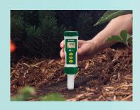
Rugged waterproof (IP57) housing with Flat Surface Electrode for measuring pH in liquids, semi-solids, and solids. Does not break or get junctions clogged like the traditional glass bulb electrodes. Easy to replace sensor is perfect for field or lab use.
