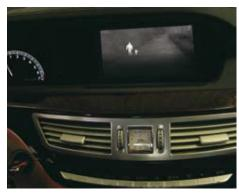
The thermal images generated by the PathFindIR can be displayed on any multi-function LCD display that accepts composite video. In this case on an LCD integrated in the Mercedes dashboard
