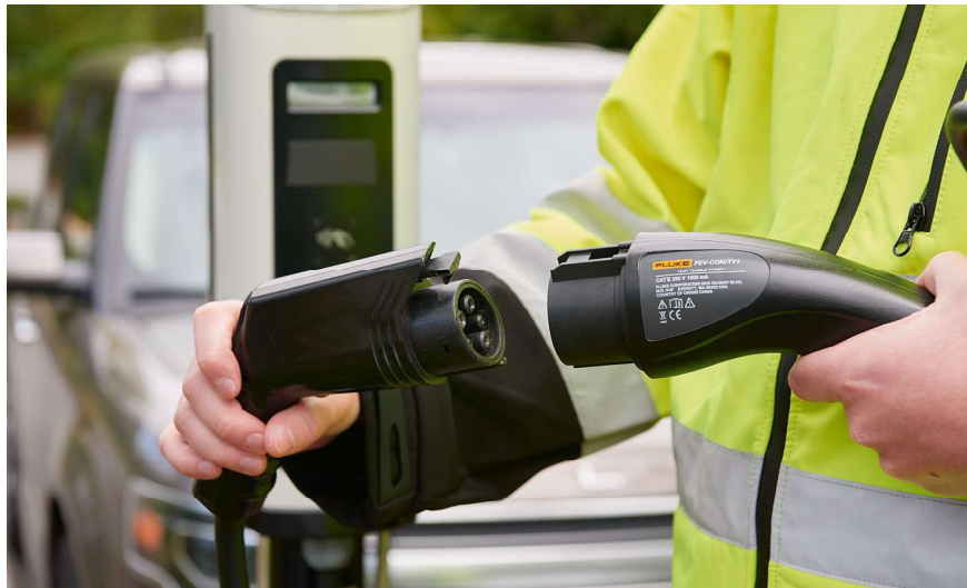
New tools like the Fluke FEV100 EVSE Test Adapter can make EVSE maintenance and troubleshooting safer, easier, and faster.
