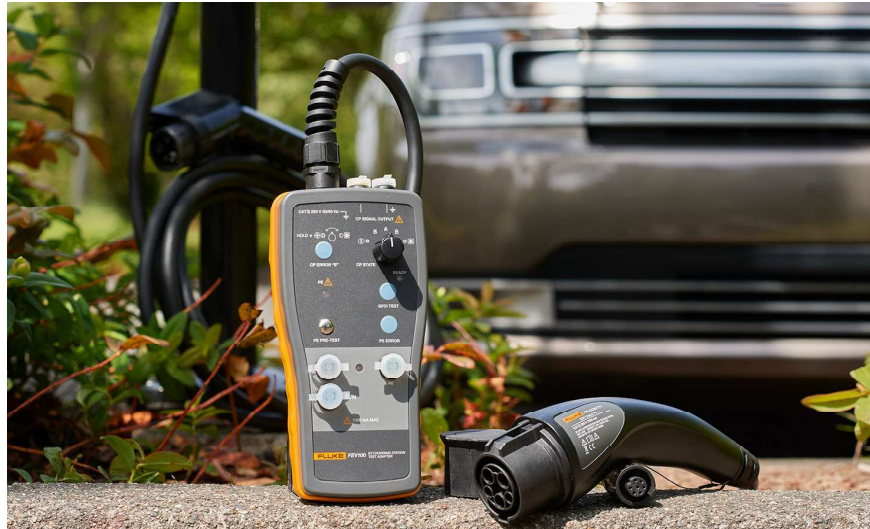
The Fluke FEV100 lets a technician test an EV charging station without an EV.
