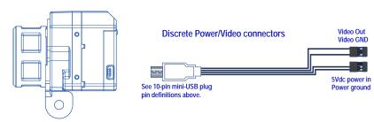
Simply plug the chosen cable into the mini-USB port on the FLIR Vue, connect the power plug to an appropriate regulated power supply, and the video plug to the video transmitter.
