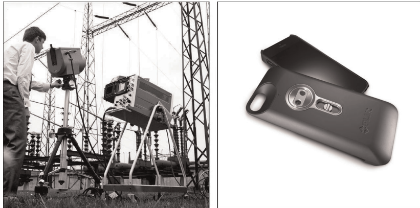
Figure 12.2 LEFT: Thermovision Model 661 from 1969. The camera weighed approximately 25 kg (55 lb.), the oscilloscope 20 kg (44 lb.), and the tripod 15 kg (33 lb.). The operator also needed a 220 VAC generator set, and a 10 L (2.6 US gallon) jar with liquid nitrogen. To the left of the oscilloscope the Polaroid attachment (6 kg/13 lb.) can be seen. RIGHT: FLIR One, which was launched in January 2014, is a slide-on attachment that gives iPhones thermal imaging capabilities. Weight: 90 g (3.2 oz.).
