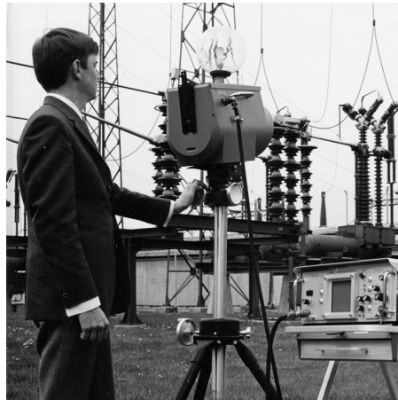
Figure 19.2 1969: Thermovision Model 661. The camera weighed approximately 25 kg (55 lb.), the oscilloscope 20 kg (44 lb.), and the tripod 15 kg (33 lb.). The operator also needed a 220 VAC generator set, and a 10 L (2.6 US gallon) jar with liquid nitrogen. To the left of the oscilloscope the Polaroid attachment (6 kg/13 lb.) can be seen.
