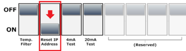
Figure 7: Set the IP reset DIP Switch to ON
