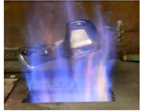
The NFPA 1801-2013 has durability requirements to help ensure that TICs are fit for fire ground duty. From left to right: durability test (tumble test), impact acceleration resistance test (drop test) and heat & flame test.
