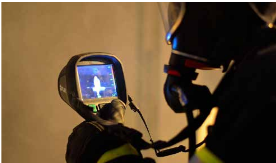
A thermal imaging camera should be easy to operate with a gloved hand.
