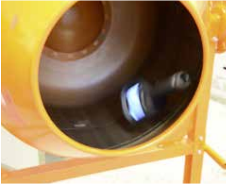
The NFPA 1801-2013 has durability requirements to help ensure that TICs are fit for fire ground duty. From left to right: durability test (tumble test), impact acceleration resistance test (drop test) and heat & flame test.
