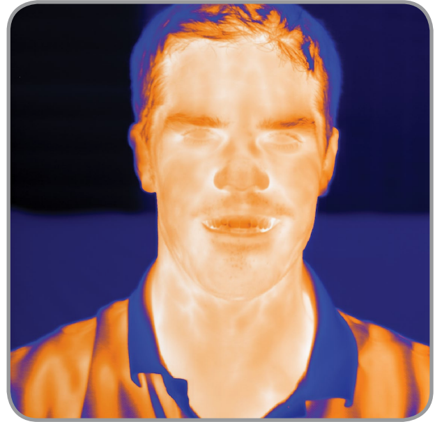
Figure 12. IR image from a 1024 × 1024 InSb detector camera
