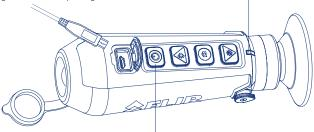
**Turning On/Off** – Press the power button to turn on your SCOUT -TK. The Indicator LED is illuminated when power is applied. The FLIR logo is displayed in the eyepiece followed by the live image. To turn OFF press and HOLD the power button. The camera shuts off after one second.
