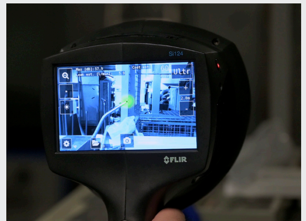
Compressed air leak detection with FLIR Si124 acoustic imaging camera
