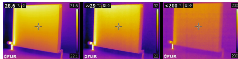
Figure 34.4 Images from a FLIR T440 with temperature ranges of -20 to +120^{\circ}\text{C} , (left, -4 to +248^{\circ}\text{F} ), 0 to +650^{\circ}\text{C} (middle, +32 to +1202^{\circ}\text{F} ) and +250 to +1200^{\circ}\text{C} (right, +482 to +2192^{\circ}\text{F} ). All other settings are unchanged.
