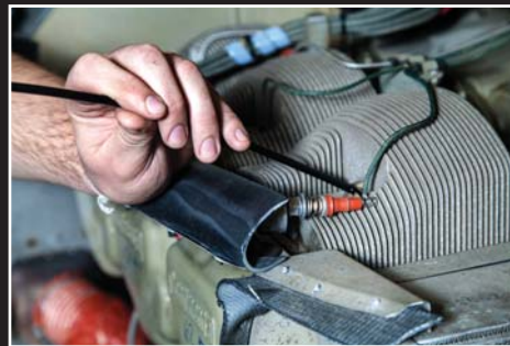
Inspecting cylinder in aircraft motor with VSA2-1M
