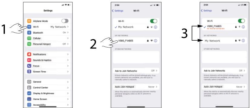
Figure 12.3 Smart device setup example. Step 1, tap the Wi-Fi setting on your smart device. Step 2, tap the VS80 from the list of available networks. Step 3, note that the VS80 is now the connected network and your personal network ('My Network', in this example) is now in the available network list, but it is no longer connected. To return to your network, simply tap your network name from the available networks (the VS80 will disconnect).
