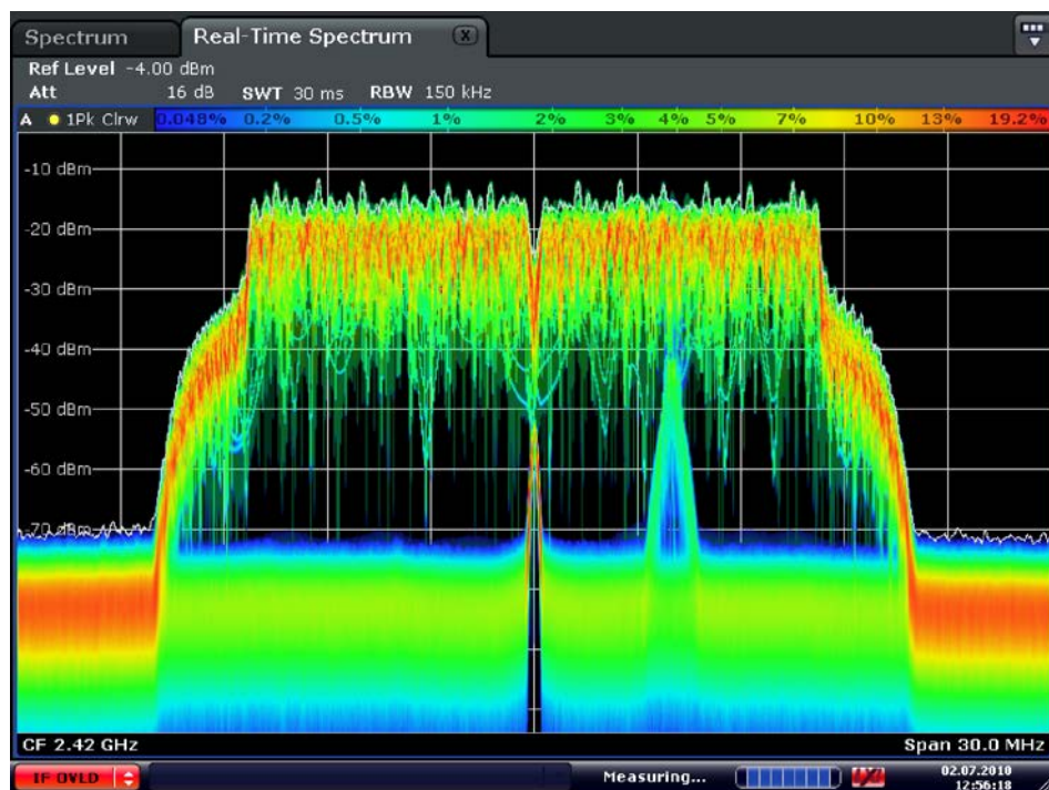
Fig. 5-16: WiFi Signal with Bluetooth Signal
