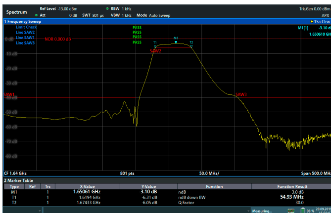
Measurement and qualification of a SAW filter (n-dB down bandwidth, quality factor)
