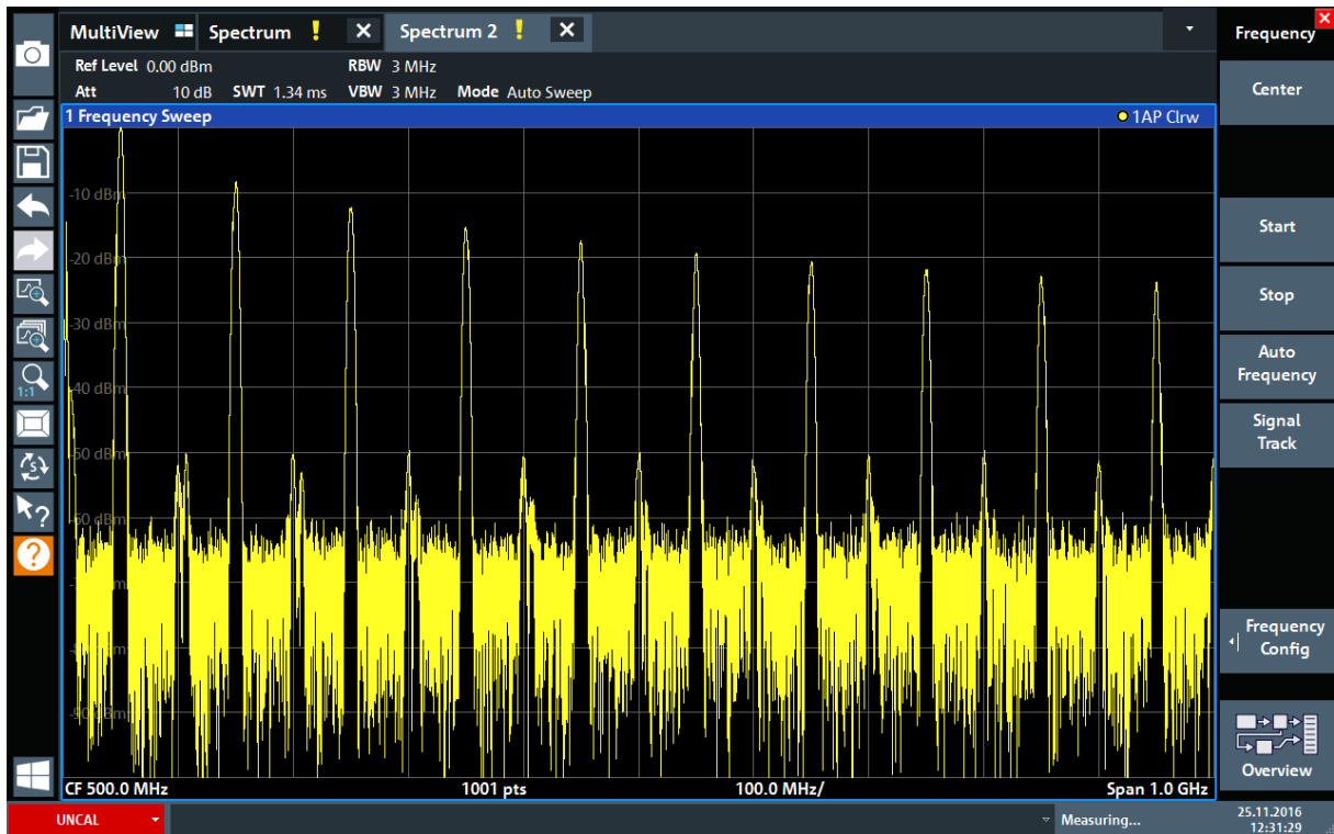
Figure 6-6: Frequency spectrum of the calibration signal with a larger span
