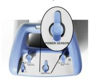
The connector is configured especially for power sensors. It is used for both the power supply and data transfer via the power sensor interface.
