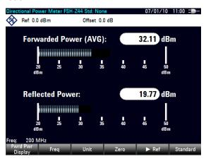
To get the best results, you should also define the frequency of the signal. For more information see "Measuring the Power with a Power Sensor" on page 65.
