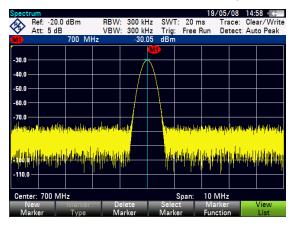
A blue vertical line represents the position of the marker on the horizontal axis (e.g. the frequency).
