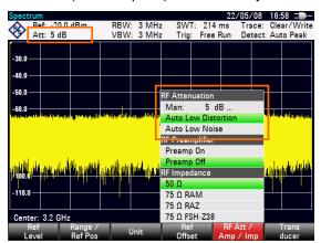
You can also set the attenuation manually. The R&S FSH provides attenuation in the range from 0 to 40 dB in 5 dB steps.
