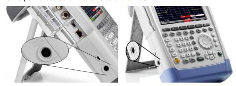
The R&S FSH is supplied with power by the AC/DC transformer power supply via the DC connector. You can also use the DC connector to charge the battery.
