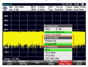
The magnitude of amplification depends on the reference level. This coupling to the reference level makes sure that the dynamic range is at an optimum.
