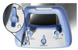
The internal impedance of the connector is approximately 10 Ohm.
