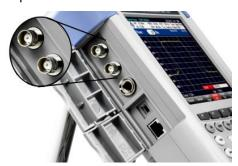
You can configure both BNC connectors for various applications. The name of the connector is printed on the insides of the protective caps.
