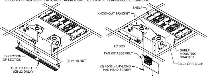
INSTALL (2) #8-32 x 1/4"-LONG PAN HEAD SCREW INTO FAN MOUNTING BRACKET (2 TURNS ONLY). PUSH FAN KIT ASSEMBLY TO TOP SURFACE OF CEILING BOX.
