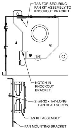
2. (a) ROTATE FAN KIT ASSEMBLY AS SHOWN. (b) SLIDE PLATE DOWN INTO NOTCH OF KNOCKOUT BRACKET. (c) ROTATE ASSEMBLY AS SHOWN SO TABS OF THE KNOCKOUT BRACKETS SLIP THROUGH THE OPENINGS ON THE FAN MOUNTING PLATE.
