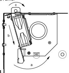
3. SECURE FAN KIT ASSEMBLY TO KNOCKOUT BRACKET WITH (2) #8-32 x 1/4"-LONG PAN HEAD SCREW.
