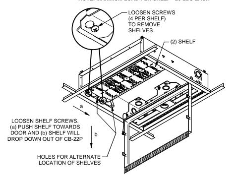
7b. FOR 1RU x 19" EIA RACK-SIZED ELECTRONICS, INSTALL RACK MOUNT BRACKETS AS SHOWN. ATTACH RACK UNIT, AND RE-INSTALL SHELF INTO CB-22P. MAKE ELECTRICAL CONNECTIONS AS REQUIRED.
