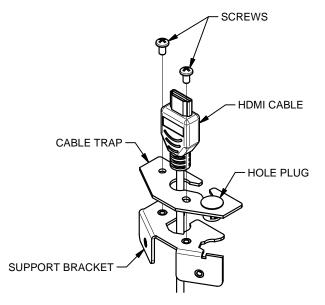
4. REINSTALL CABLE-PULL ASSEMBLY AT INDICATED HOLES.
