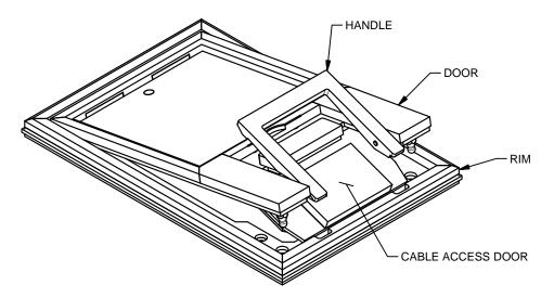
4. INSTALL RIM WITH SUPPLIED FLAT HEAD SCREWS. REVERSE DOOR REMOVAL STEPS TO REINSTALL DOOR AND PUSH FIRMLY ON HANDLE-END CORNERS TO SNAP DOOR SECURELY IN PLACE. INSTALL FINISHED FLOORING MATERIAL.
