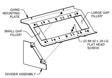
\* GAP FILLERS ARE OPTIONAL. PER DESIRED CONFIGURATION (SEE PREVIOUS PAGE), AND ARE INSTALLED SIMILARLY TO DIVIDER ASSEMBLIES
