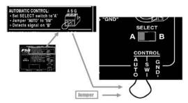
Normally "sees" Input "A" and switches to Input "B" when a video signal is present on "B"
