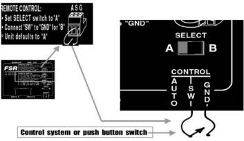
Maintained contact closure from an external switch or relay.
